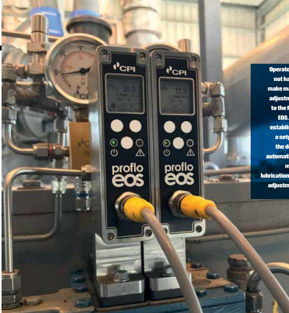
**Operators do not have to make manual adjustments to the Proflo EOS. After establishing a setpoint, the device automatically makes lubrication level adjustments.**
