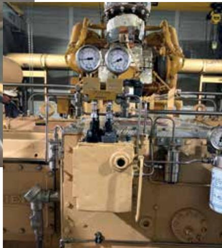
**In this photo, a gearbox is fitted with a manual lubrication pump. The Proflo EOS can make automatic adjustments.**
